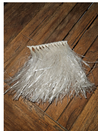
Figure 1. Biogrow Media Used in Wastewater Treatment
