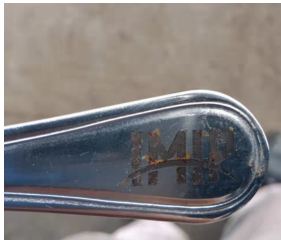
Figure 2. Sample Stainless Steel 304L After Corrosion
