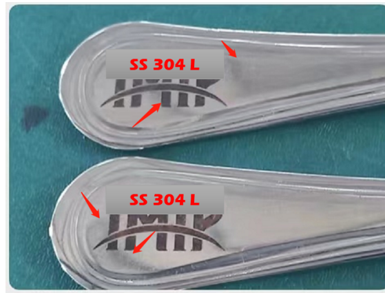
Figure 1. Sample Stainless Steel 304L Before Corrosion
